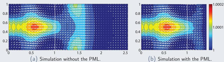
Figure 2: Density distribution and velocity field at  $t = 1.00$ .
